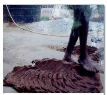
**Figure 14a.** Kaolinite clay can be made more pliable by wedging, where it is rolled into a tight spiral with a sort of kneading method, which removes air pockets. Source: Lalita Manjunath.
