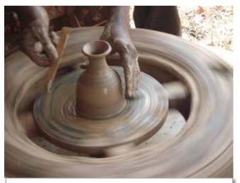
**Figure 14c.** The small amount of water that enters clay allows it to be moulded into pots. Source: Lalita Manjunath.
